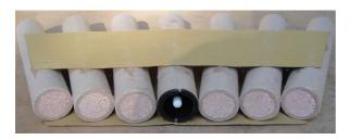
\* STEP 2. Foil is taped over the fusing to minimize internal crossfires with the next row of modular. No unexpected firings at the wrong time!
