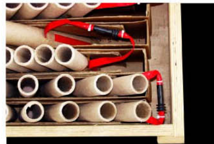
Individual Modules linked together using the Fire Transfer Connectors
