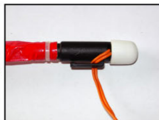
Electric Match inserted and covered with Cap
